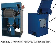
7.5 H.P TEFC Motor is standard 230/460 /3 phase /60 cycle
