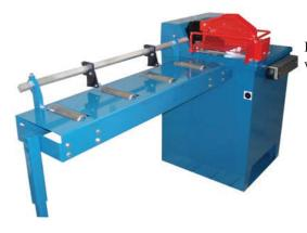
Roller Infeed and Outfeed Tables with a Gauge Bar and Stops
