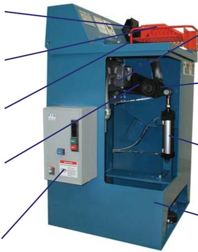
7.5 H.P TEFC Motor is standard 230/460 /3 phase /60 cycle.
